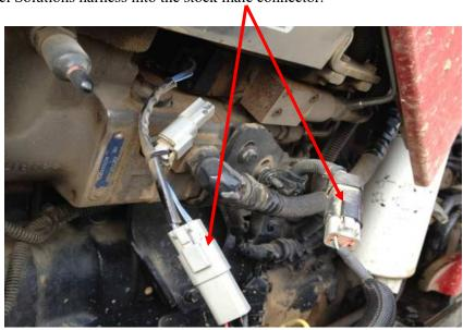
**4)** Unplug the MAP Sensor. Plug the male MAP sensor connector from the Ag Diesel Solution harness into the stock female MAP sensor connector.
