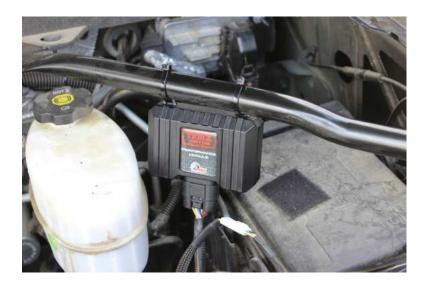
8) Once you have installed the module, connect the switch to the switch pigtail. Once connected you can zip tie it to the module and leave it in place.
