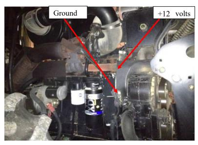
**12)** Mount the module with the connector on the bottom side, as to reduce the chance of moisture from getting into the module harness. Keep away from excessive heat and moving parts.
